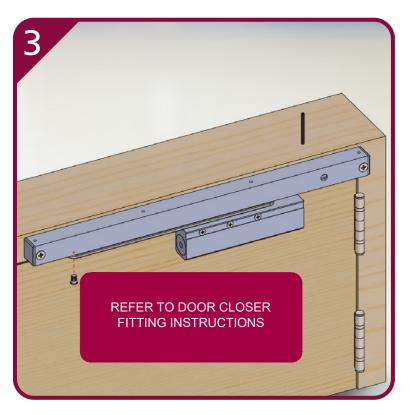
MPORTANT NOTES: THE PINION BOLT MUST BE TIGHTENED TO 12Nm.
