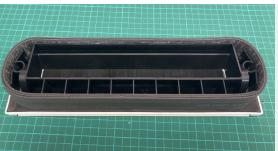
Continue to stick the intumescent around the letterplate as shown in picture. There must be three layers of intumescent covering the bottom ribbed section
