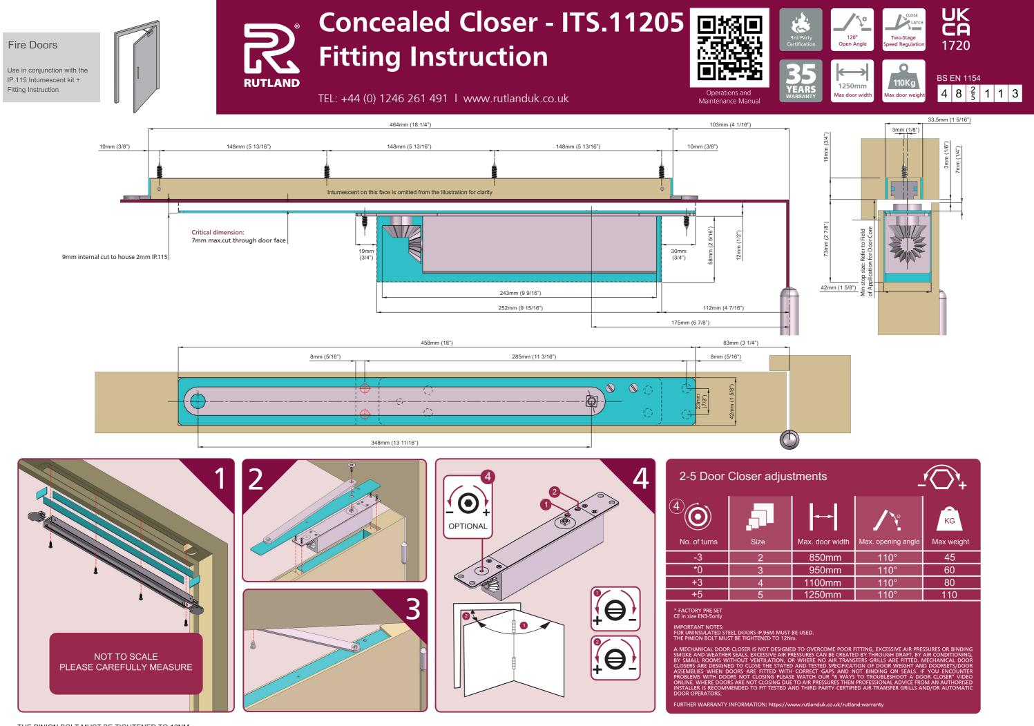
THE PINION BOLT MUST BE TIGHTENED TO 12NM FIRE DOORS MUST BE FITTED WITH INTUMESCENT GASKETS
