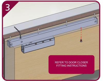
MPORTANT NOTES: THE PINION BOLT MUST BE TIGHTENED TO 12Nm.
