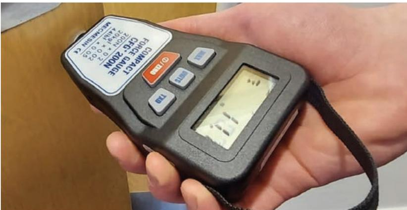
In simple terms, door opening and closing forces are measured with a force gauge, of one sort or another. For accurate measurements, an electronic force gauge is recommended, and these can be fitted with different attachments to measure push or pull force. Routine calibration is required to ensure that measurements remain accurate.
