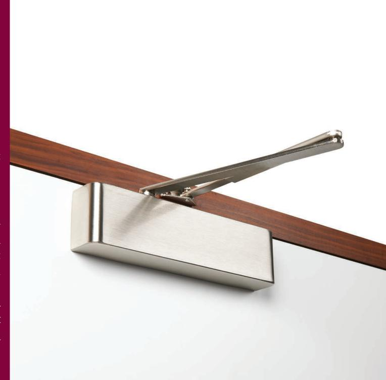
TS.9206 is ideal for heavy usage and is power adjustable by spring size 3-6. This closer has a unique slimline appearance and comes with back check and delayed action as standard.
